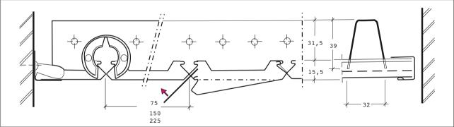
Carrier for panels 32 mm wide, 39 mm high. Produced from aluminium thickness 0,95 mm or thickness 0,65 mm in steel.
